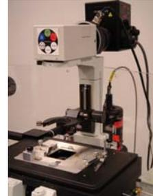
7. Remove Temperature controller from the chamber, install it next to the microscope base. Remove temperature control sensor from plastic bag secured on the top of temperature controller, and install it on the microscope pillar.
