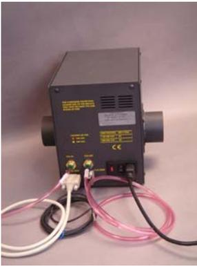
14. If applicable, connect CO2 tube to push to release connector marked "CO2 Port 1" on the back of the chamber.
