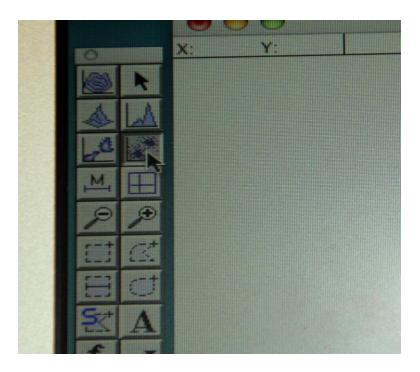
Setting up instrument settings for FSC, SSC, FL1-FL3 Go to Cytometer menu- instrument control. By clicking on the axis of the Plots and using the menu to the right you will be able to assign the parameters you would like to measure.
