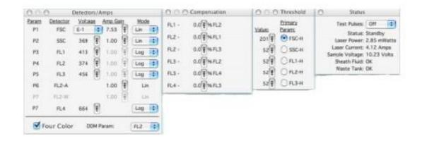
Adjust the FSC amplifier, SSC detector in detector/amps window to find your populations of cells.
